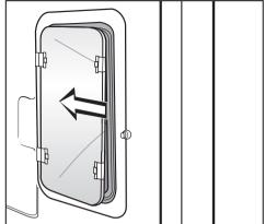
■ Put the light cover back in place with the notch to the rear of the metal clamps.
